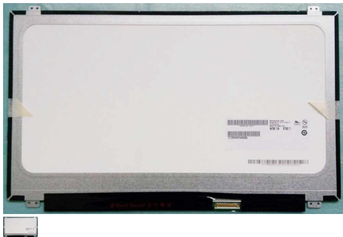
Display LCD portátil 15.6" Model: B156XTN03.1 Slim special 30 pins
